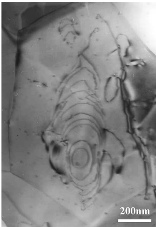
Fig. 11 Bright field image showing the dislocation loops
